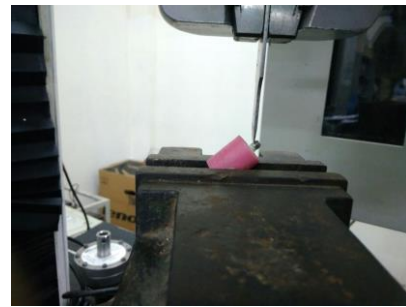
Figure 1: Fracture resistance testing under universal testing machine
